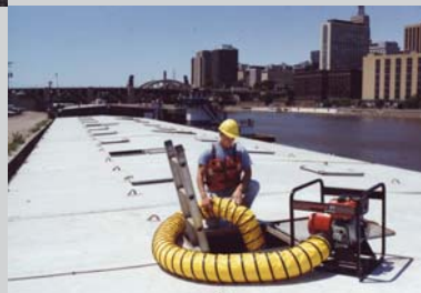
DP8 , 5 1/2 HP, diesel, radial airflow
