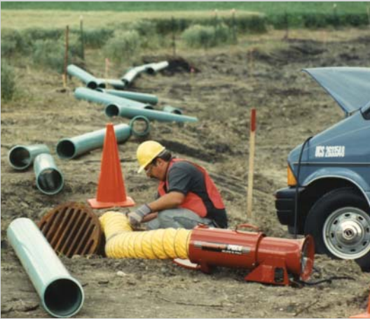
EP8DC15 , 1/6 HP, 12 VDC, axial airflow
