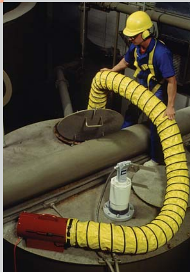
EP8AC , 1/4 HP, 115 VAC, axial airflow
